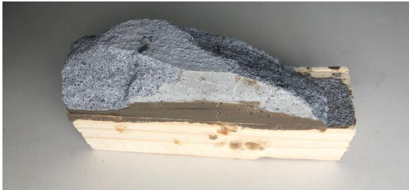
Figure 4.5 Failure mode of concrete failure.
