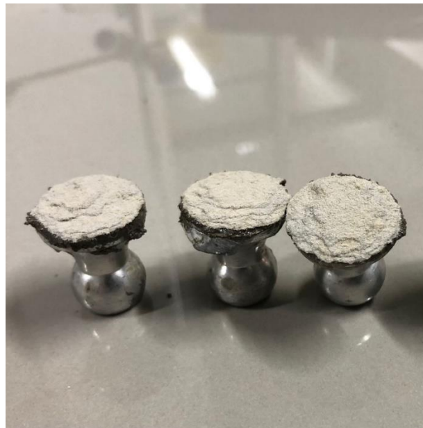
Figure 4.1 Failure modes of the pull off test specimens.
