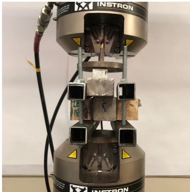
Figure 3.8 Setup for the double lap shear test.
