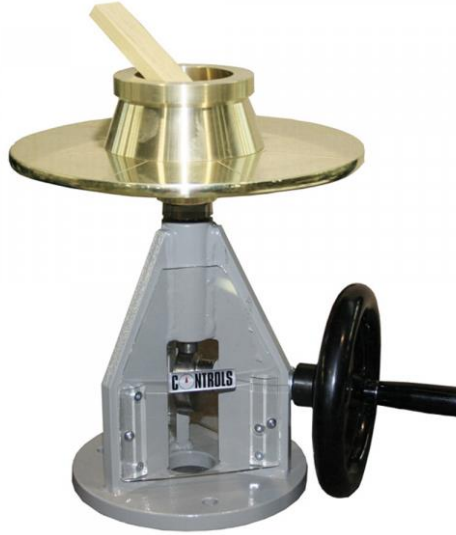
Figure 3.1 Flow test table setup.
