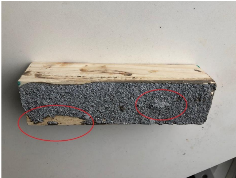
Figure 4.4 Failure mode of removal of the facial cover. It can be appreciated in the red circles the variety of failure along the whole piece.
