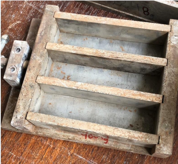
Figure 3.3 Steel molds for 40x40x160mm pieces.
