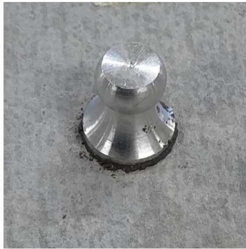
Figure 3.6 Bearing ring glued to the fibre cement plate.
