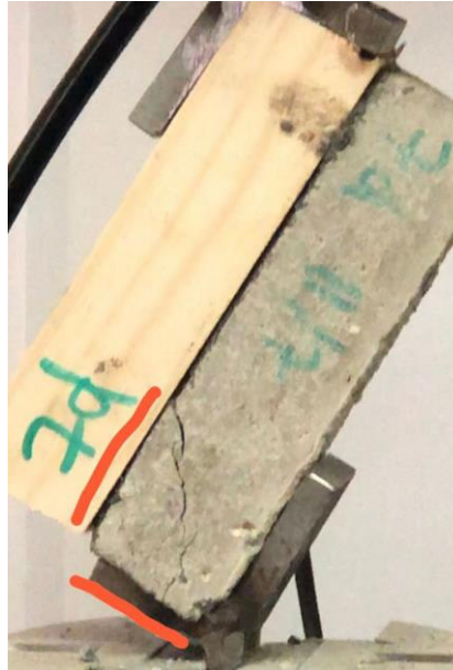
Figure 4.3 Fracture lines in the test.
