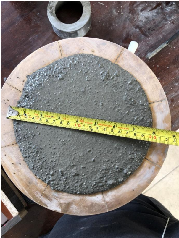
Figure 3.2 Concrete mix after applying the flow test
