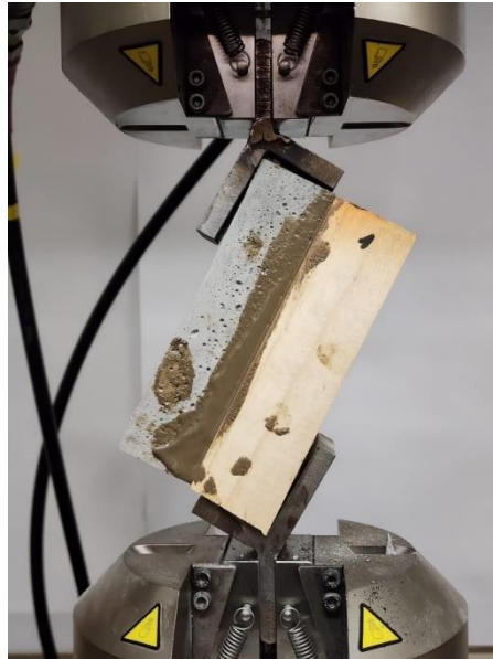
Figure 3.7 Specimen of a compression-shear test.
