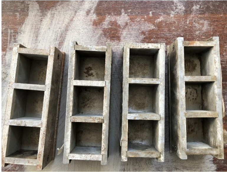
Figure 3.4 Steel molds for 50x50x50mm pieces.
