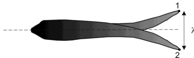
Figure 3.3 Digitized points for determination of the tail beat amplitude \lambda
