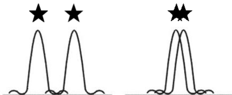
Figure 6: A graphic explanation of how determining a good Point Spread Function can characterize the light profile of stars in crowded fields. Source: Own elaboration
