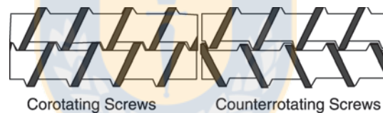
FIGURE 2.2: Co-rotating and counter-rotating twin-screws [7].
