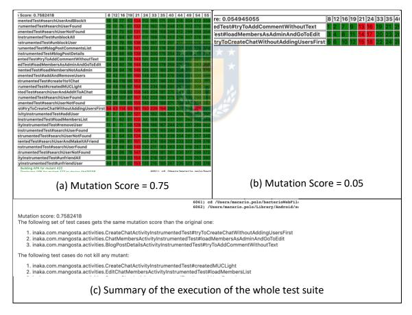
Figure 58. Reducing the test suite does not always produce reliable results
