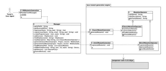
Figure 28. Decoupled design of the mutant generation engine
