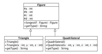
Figure 25. A simple system with inheritance
