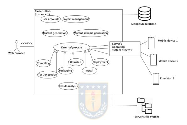
Figure 12. General structure of BacterioWeb v.1
