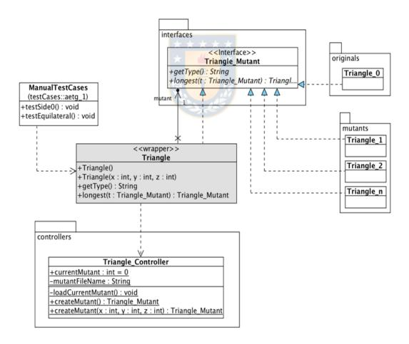
Figure 17. Final structure of the Mutant Schema
