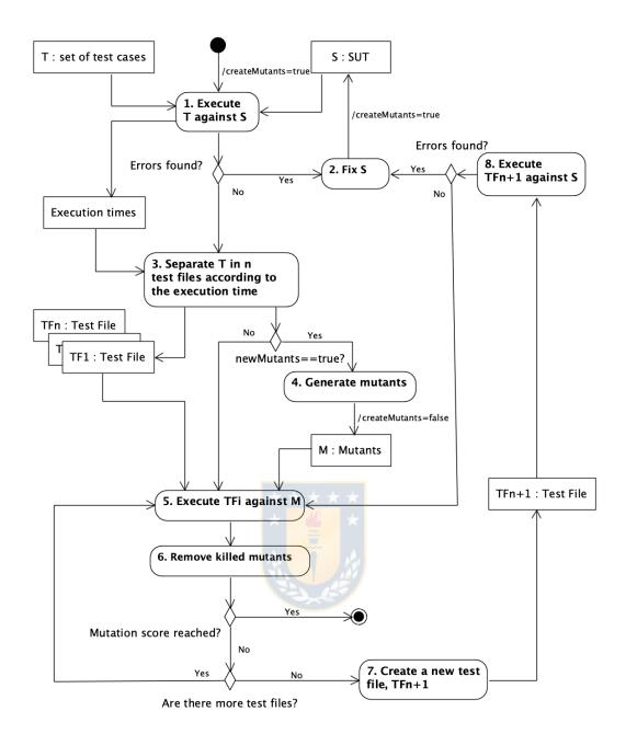
Figure 59. A mutation process, specifically adapted to mobile software
