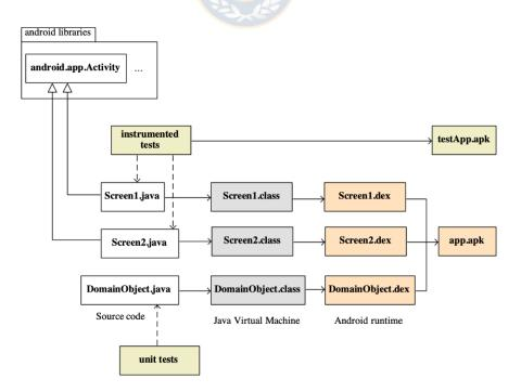
Figure 4. Compilation and packaging of an Android app
