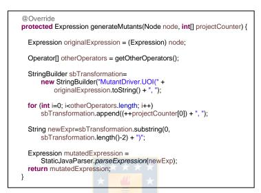
Figure 30. Implementation of the UOI operator in Untch's
