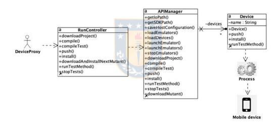
Figure 47. Connection between a *DeviceProxy* (on the CWS) and its physical device (on the DWS)
