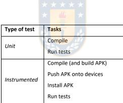
Table 13. Execution tasks depending on the type of tests
