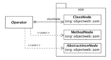
Figure 11. Dependencies of our Operator with respect to ASM
