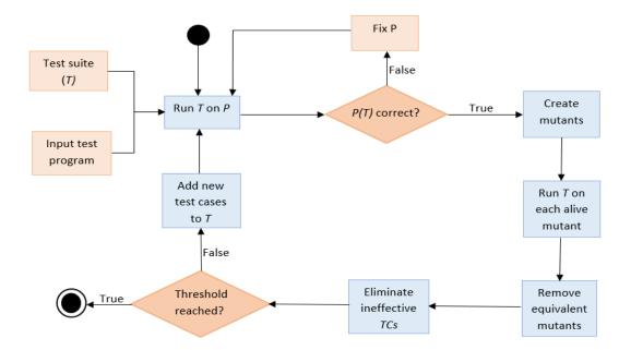
Figure 1. "Traditional mutation testing process", where T is the test suite and P is the program under test and TC is a test case
