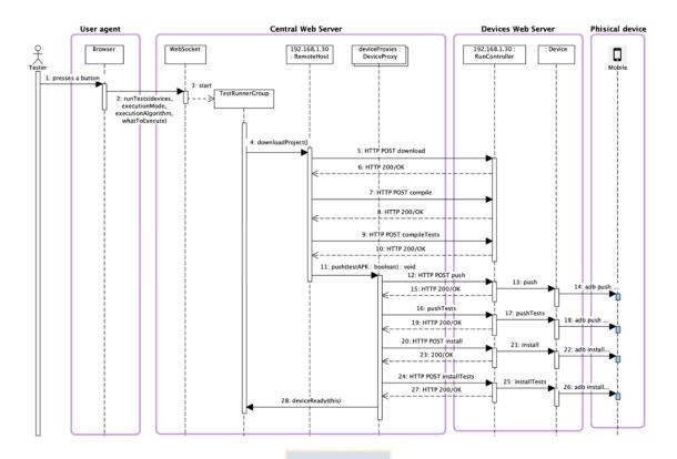
Figure 45. Sequence of operations for starting a test execution
