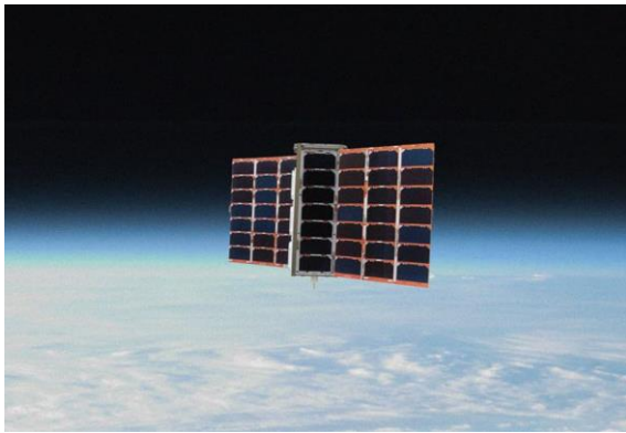
a) Low Earth Multi-Use Receiver (LEMUR) 3U CubeSat de Spire Global (Spire Global)
