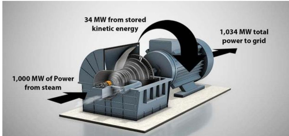
Figura 2.2 Source of power in a 1000 [MW] contingency case with 29 identical 1000 [MW] generators [3].
