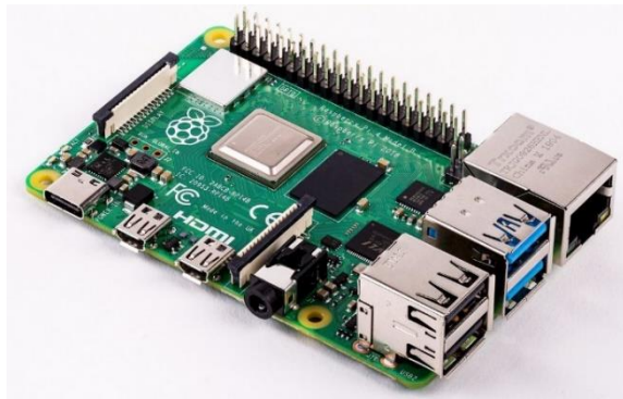
Fig. 6.8. Microcontrolador Raspberry Pi 4.
