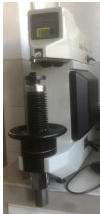
Figura 31. Macro durometro Roell ZHR, Zwick.
