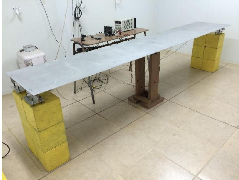
Figure 3.3 Laboratory scaled bridge model on climate chamber.
