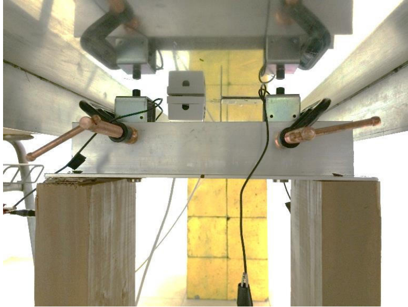
Figure 3.4 Solenoids excitation system at middle span.
