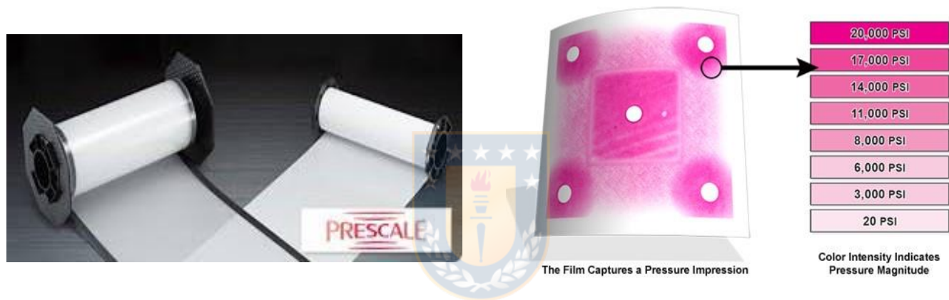
Figure 8. Fujifilm's Prescale pressure measurement film (source: [ https://www.fujifilm.com ]).
