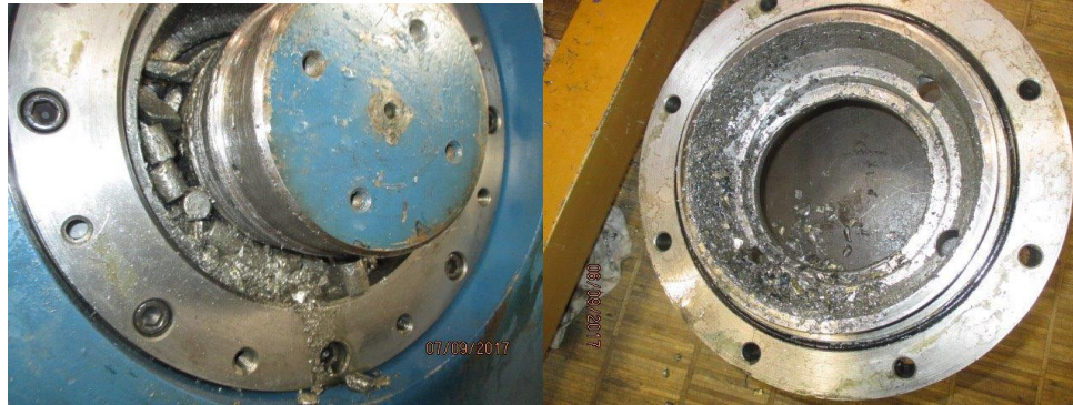
Figure 5. Bearing damage, UT4-RTM 2 (source: [ESO Workshop Paranal 2017]).
