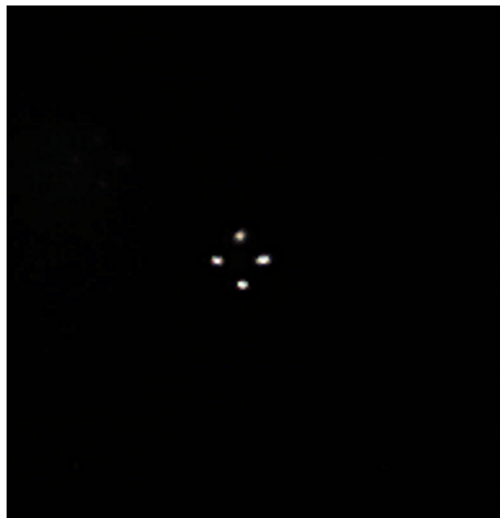
Figure C.4: 4-Core image camera. Optical image of multicore fiber and used for analysis. Source: Made by author.
