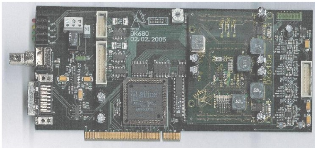
Figura 7: Tarjeta IRIG-B/Blank-Sync. (Fuente: Bernd Klein (2007). “CSO-FFTS A fast fourier transform spectrometer for the CSO”[8].)
