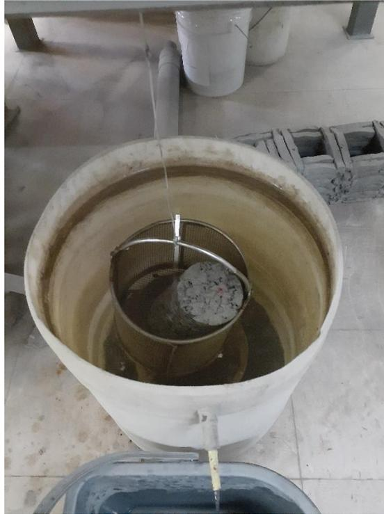
**Figura 3.8. Probeta sumergida**
