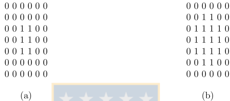
Figure B.6: Dilation of a rectangle: An image with a small rectangle (a) and its dilation (b) with the 3x3 cross.
