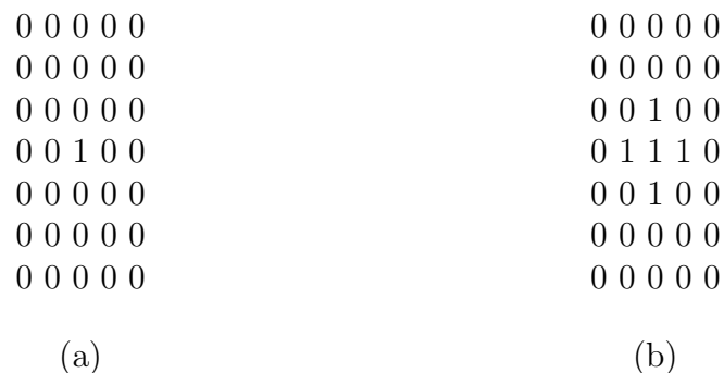
Figure B.5: Dilation of a pixel: An image with a pixel (a) and its dilation (b) with the 3x3 cross.
