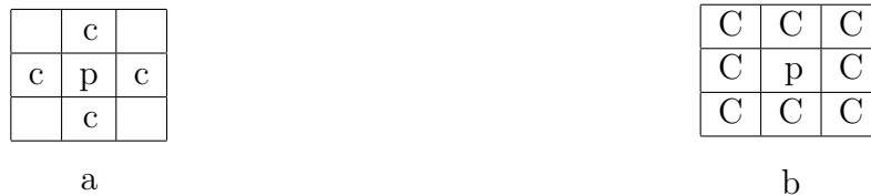
Figure A.7: Neighbors of a pixel: (a) 4-neighbor and (b) 8-neighbor pixels of p
