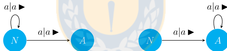
Figure 3.3: Graph representation of \delta (left) and \delta' (right) of non-deterministic machine M = (\{N, A\}, \{a, b\}, \delta) and deterministic machine M' = (\{N, A\}, \{a, b\}, \delta') accepting a^+ . The machine accepts the input when it halts in state A .
