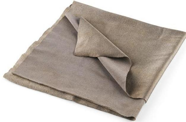
**Figura 3.2 Tela conductora Shieldex.**
