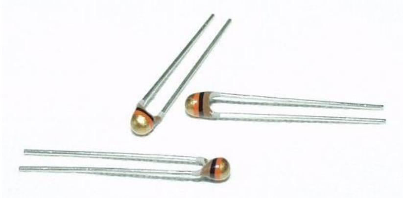
Figura 3.5 Termistor 10[k $\Omega$ ] NTC.
