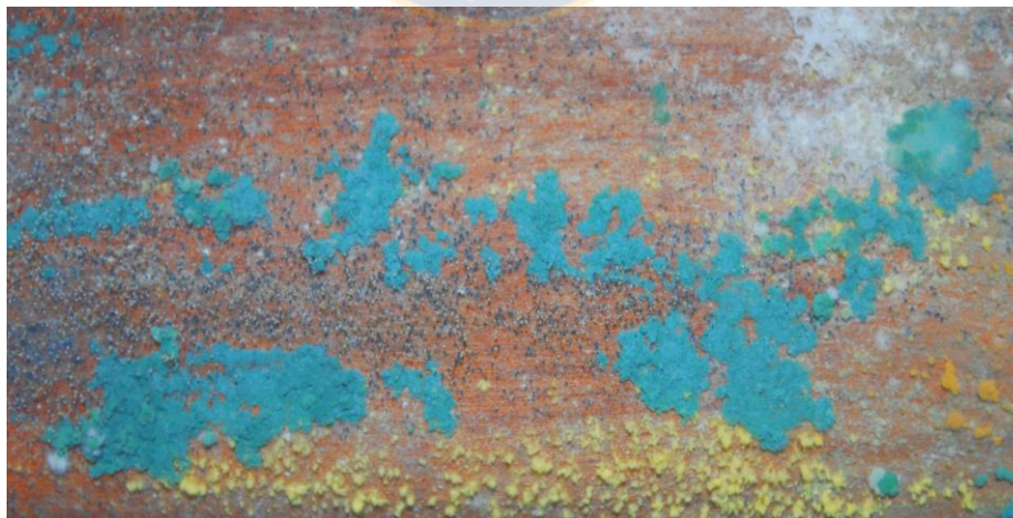
Figure 3: Colonization and growth of fungal structures after mixed cultures of Ophiostoma sp, Eurotium sp. and Phialocephala sp. were applied on Nothofagus obliqua .
