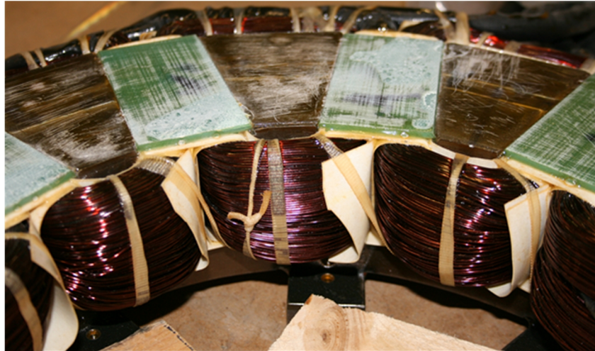
Fig. 4.19. Stator core with a double-layer TCW. (Jara et al., 2016)
