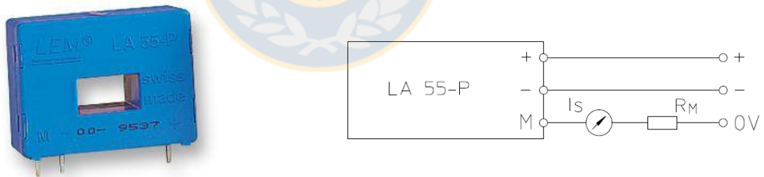
Fig. 4.12. Current transducer LA55-P and its connection
