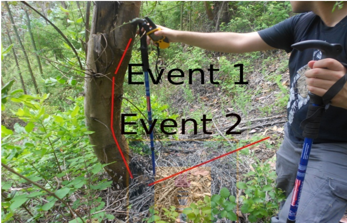
Figure 2.8 Bent tree log due to progressive soil deformation. Source: Fustos et al., 2017.
