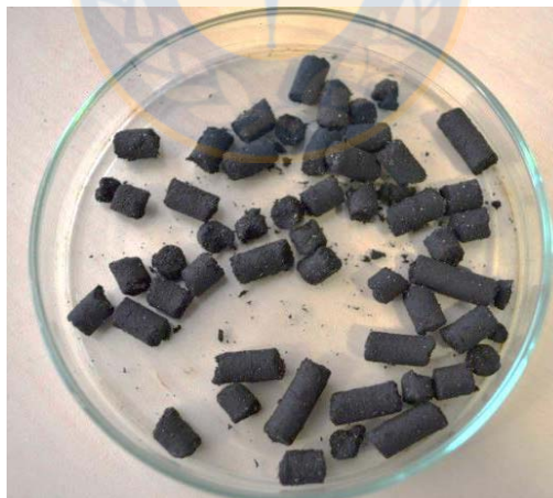
Figure 2.1. Cylindrical aspect of manufactured pellets for compress with ash and sludge from a paper mill.
