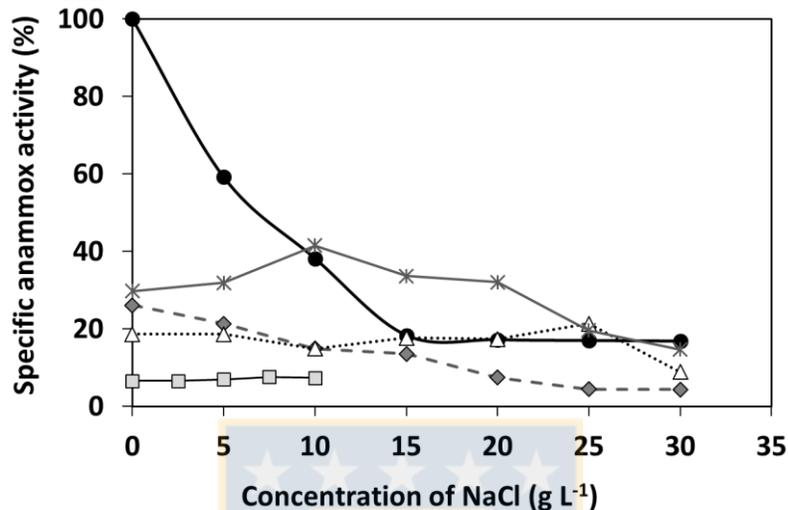
**Figure 5.4:** Percentage of remaining SAA in the assays with the salt concentration for the SBR biomass on different operational days: inoculum (●), Stage A-IV on day 142 (■), Stage-B on days 11 (◆), 31 (△) and 39 (\*). The values correspond to average values of the experiments performed in triplicate (standard deviation lower than 10%).
