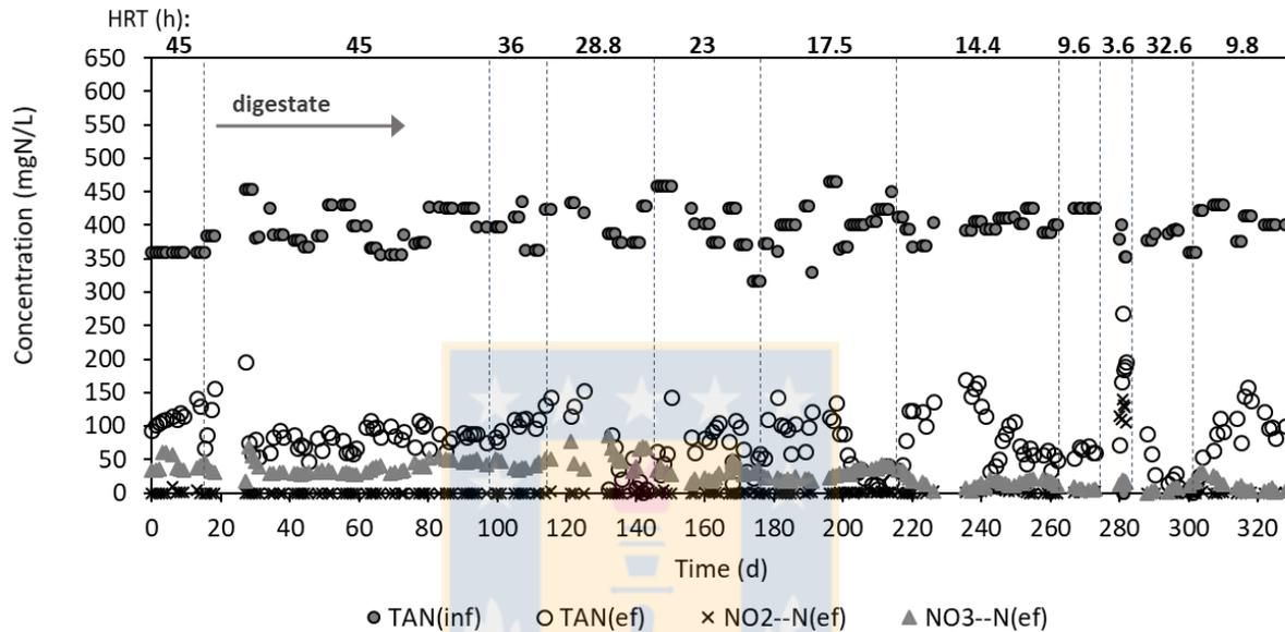
**Figure 4.1:** Nitrogen compounds profile in the different operational stages with HRT from 45 to 3.6 h. TAN in the influent (●) and TAN (○),  $\text{NO}_2^-$ -N (×) and  $\text{NO}_3^-$ -N (▲) in the effluent. Grey arrow indicates the change of synthetic substrate to digested poultry manure.
