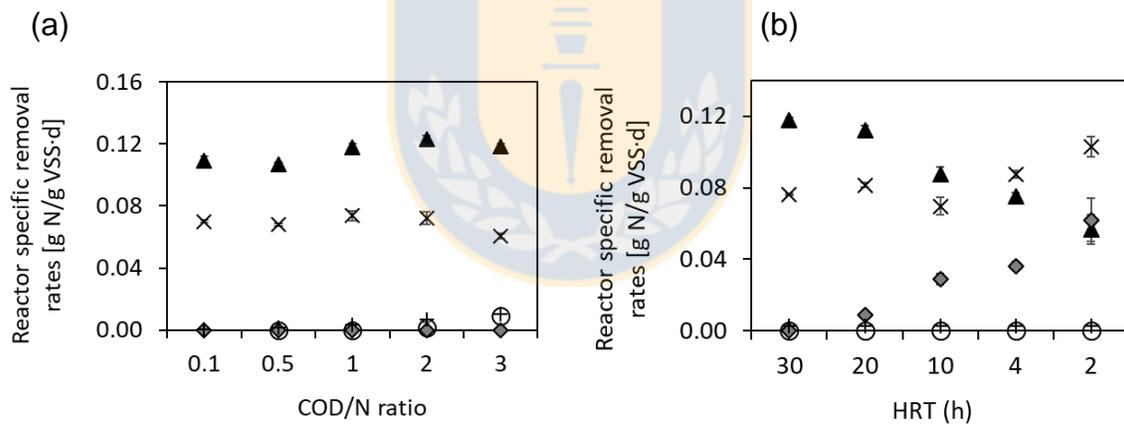
**Figure 2.2:** Reactor specific nitrogen removal rates by Anammox (AR<sub>x</sub>) (▲), ammonia oxidizing (AOR<sub>x</sub>) (×), nitrite oxidizing (NOR<sub>x</sub>) (◆), denitrifying (DR<sub>x</sub>) (○) bacteria, and heterotrophic nitrogen assimilation (HNA<sub>x</sub>) (+) obtained at constant NLR of 240 mg N L<sup>-1</sup> d<sup>-1</sup>, with: (a) different COD/N ratios at 30 h of HRT; and (b) variable HRT at COD/N ratio of 0.5.
