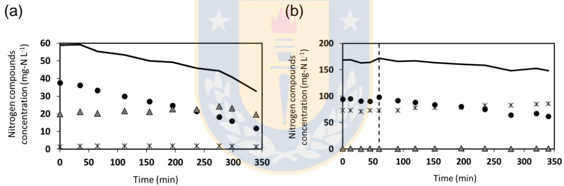
**Figure 5.2.** Evolution of nitrogen compounds concentrations inside the reactor: TAN (●), NO<sub>2</sub><sup>-</sup>-N (\*), NO<sub>3</sub><sup>-</sup>-N (▲) and TN (—), for an operational cycle: (a) Stage A-II, day 74 and (b) Stage A-III, day 130.
