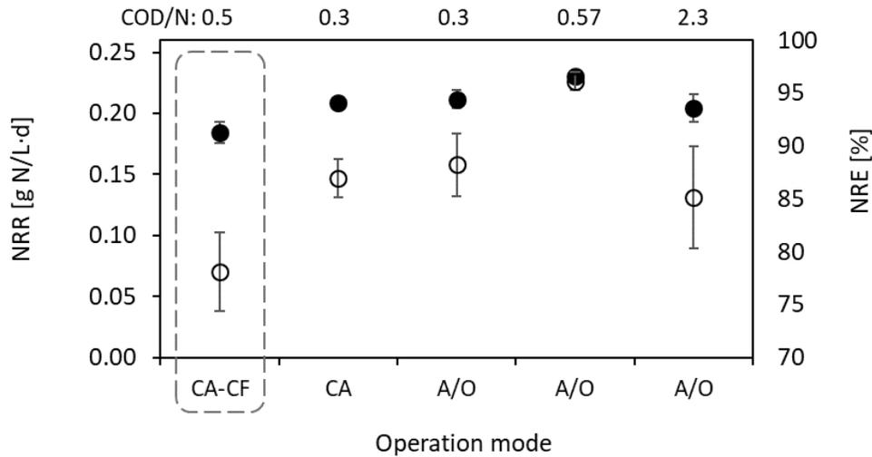
**Figure 3.2:** Nitrogen removal rates and efficiencies (NRR and NRE, respectively) obtained in the different operational stages: NRR (●) and NRE (○). COD/N: inlet COD/N ratio; CA: Continuous aeration; CF: Continuous feeding; A/O: Anoxic/Oxic operation mode; CA-CF: Experimental average data obtained with two identical reactors operated with continuous regime [30].
