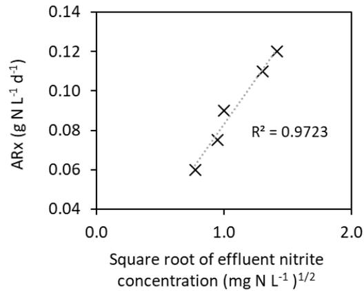
**Figure 2.4:** Correlation between specific nitrogen removal rate by Anammox ( $AR_x$ ) and the square root of the nitrite concentration ( $\times$ ) measured at the effluent of reactor 2 with variable HRT.
