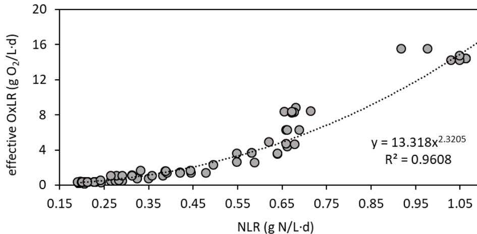
**Figure 4.4:** Effective Oxygen Loading Rate (OxLR) applied to maintain the nitrogen removal efficiency at the different Nitrogen Loading Rates (NLR) assayed in the system.
