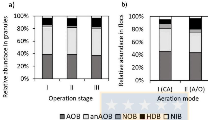
**Figure 3.5:** Relative abundance of main bacterial groups of the partial nitrification-Anammox process obtained in granules (a) and flocs (b), at different operational stages and modes. CA: continuous aeration; A/O: anoxic/oxic operation mode. AOB: ammonia oxidizing bacteria; anAOB: anaerobic ammonia oxidizing bacteria; NOB: nitrite oxidizing bacteria; HDB: heterotrophic denitrifying bacteria; NIB: non-identified bacteria.
