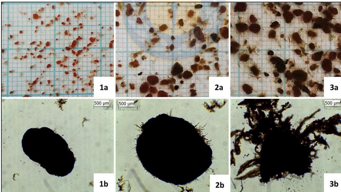
**Figure 4.3:** Granules images over millimeter paper (1a, 2a, 3a) and under optical microscope (1b, 2b, 3b). 1a,b: Inoculum granular biomass; 2a,b: Granules after 140 days of operation with digestate at 28.8 h of HRT; 3a,b: Granules after last HRT proved of 3.6 h.
