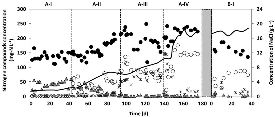
**Figure 5.1:** Profiles of salt and nitrogen compounds concentrations in the different operational stages: NaCl (—), TAN in the influent (●) and TAN (○), NO<sub>2</sub><sup>-</sup>-N (\*) and NO<sub>3</sub><sup>-</sup>-N (▲) in the effluent.
