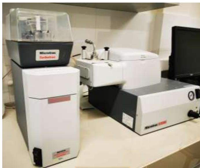
**Figura 30** Microtrac - Model S3500 – Particle Size Analyzer del Laboratorio ASIF.
