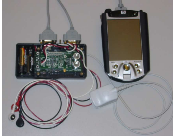
Figure 6.3: Inside the patient waist pack: SpO 2 and ECG sensors, sensor box and HP iPAQ ®.
