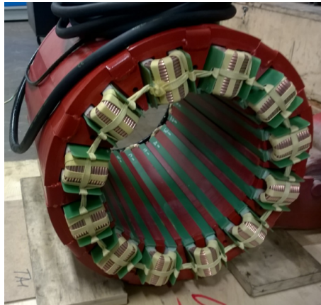
Figure 4.5: Prototype stator assembled. Glass-fibre slot keys guarantee the fixing of the coils. No impregnation was used for the winding.
