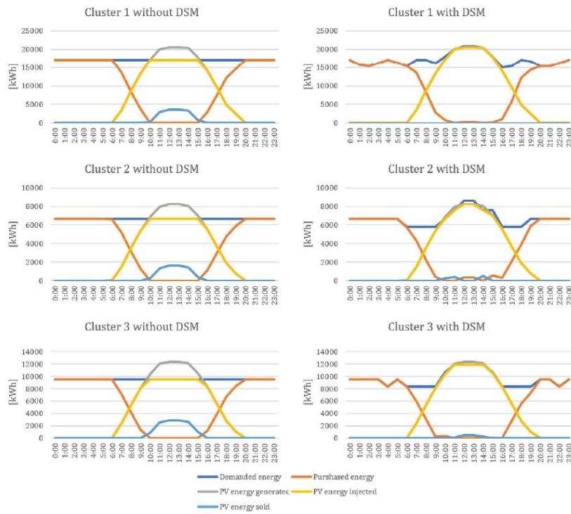
Figure 6: Energy profiles by Clusters for cases without and with DSM (month of December).
