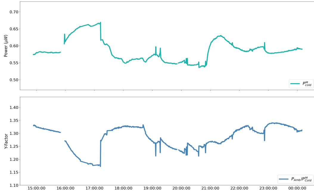
Figure 5.6.13: Y-factor of measurements (second panel) influenced by the Cold power of the calibrator immersed in LN 2 -container (first panel).
