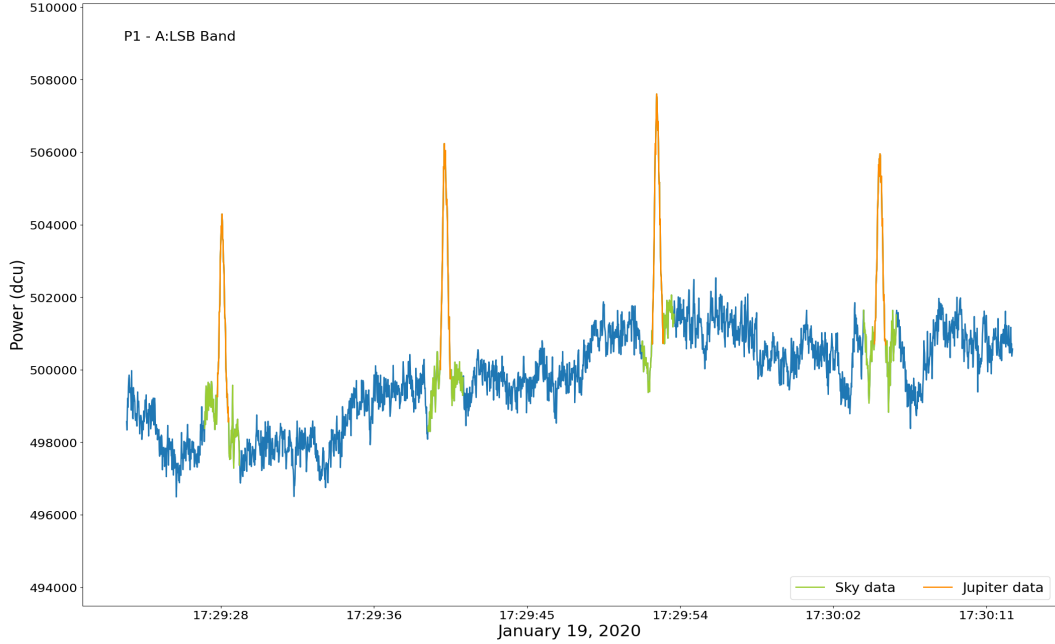
Figure 4.2.14: Power section contains Jupiter data of pixel 1, A:LSB band from obsid10611 file is shown. Jupiter’s section is shown in the orange line, and the sky’s section is illustrated in the light green line.
