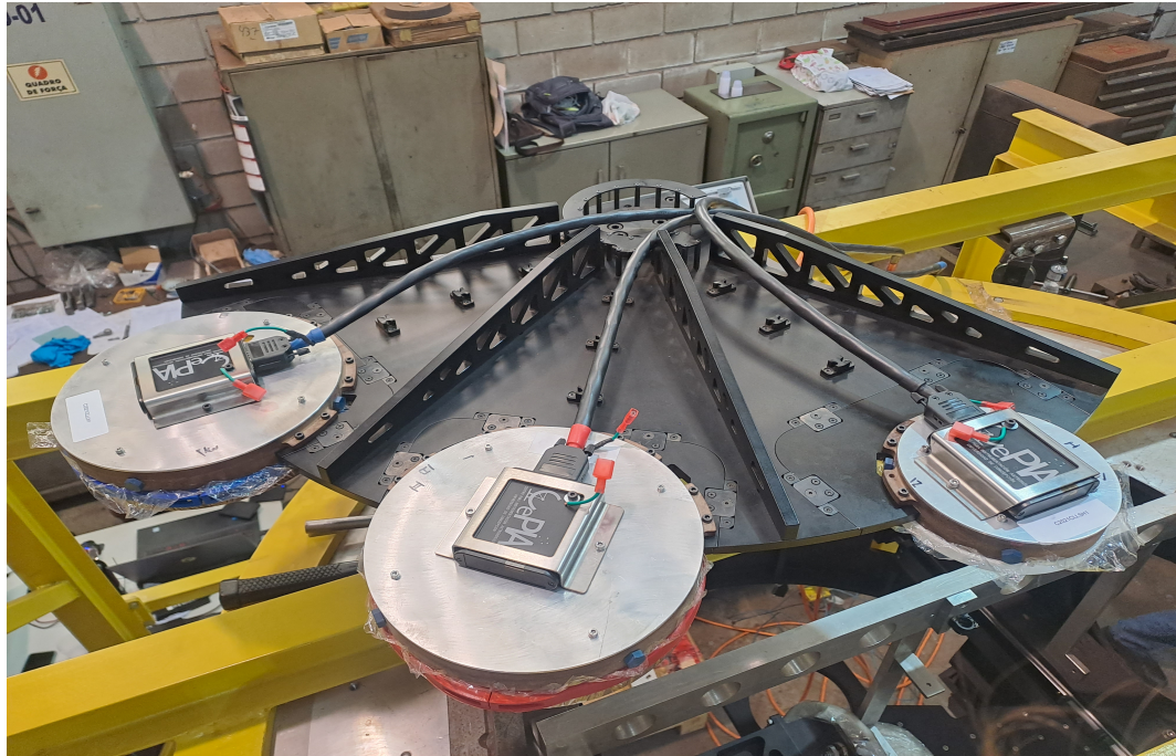
Figure 5.4.9: Final calibration loads mounted on the robotic arm of the Cassegrain cabin of the LLAMA radio telescope.
