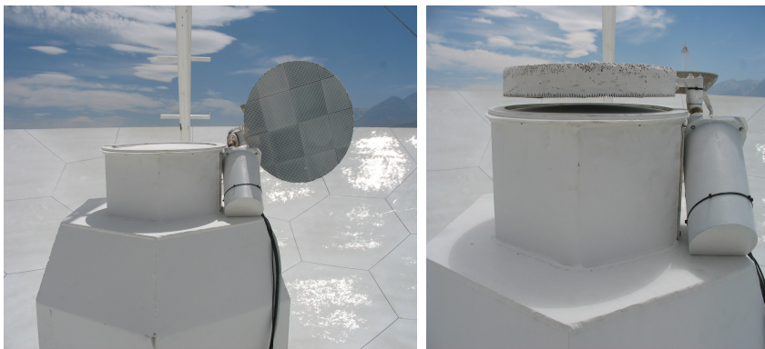
Figure 4.2.2: The calibration load is mounted on the side of the COMAP receiver. The left panel illustrates the load positioned outside the field of view of the 19-pixel array (calibration state 0.0), while the right panel displays the load placed in its calibration position (calibration state 1.0).
