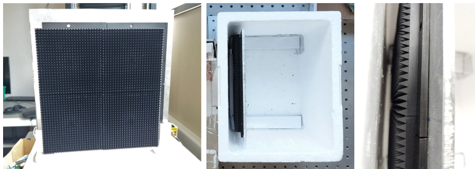
Figure 5.6.4: Calibration device based on RAM tiles. Panel 1 displays the calibrator, which consists of four RAM segments mounted onto an aluminum plate and designed to be submerged in LN2-box. Panel 2 illustrates the calibrator placement inside the expanded polystyrene container, which is pointing to the mirror. Panel 3 provides a broader view, highlighting that the calibrator does not touch the container walls, allowing the calibrator to come into direct contact with the LN2.
