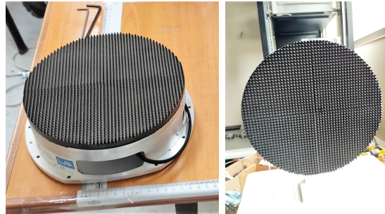
Figure 5.7.2: The ambient calibrator used to monitor ambient power during radiometric measurements is shown.
