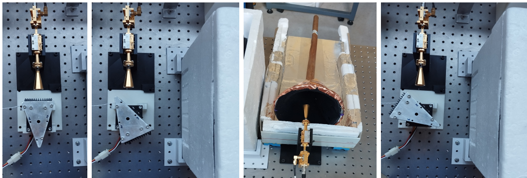
Figure 5.6.9: Different configurations of the measurement system, utilizing the three calibrators to characterize both mirror plates, are displayed. Panels 1 and 3 exhibit the direct measurements of the ambient and LN2 cone calibrators at the receiver. Panels 2 and 4 show the mirror positioned on sides 1 and 2, respectively, with the beam directed toward the calibrator within the LN2 container.
