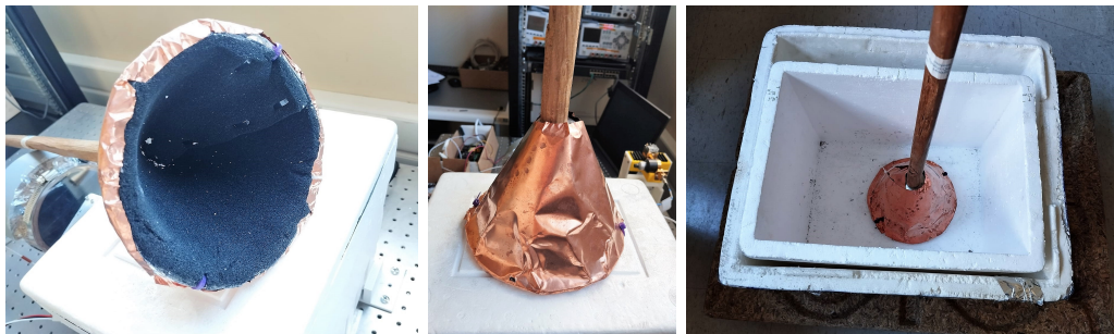
Figure 5.6.6: Liquid nitrogen direct calibration device utilized in radiometric measurements of prototype. Panels 1 and 2 present different perspectives of the direct cone employed as a calibrator, while Panel 3 displays the expanded polystyrene container designated for the LN2 containment.
