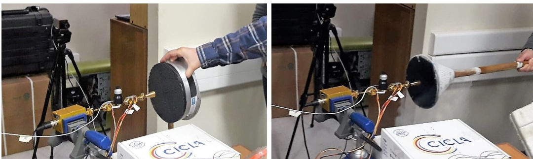
Figure 5.7.4: The calibrators used for the calibration process during power measurements of the final calibration loads set at 40°C, 50°C y 70°C are shown. The left panel presents the ambient calibrator, while the right panel displays the LN2 cone, both measured by the 93-GHz receiver.
