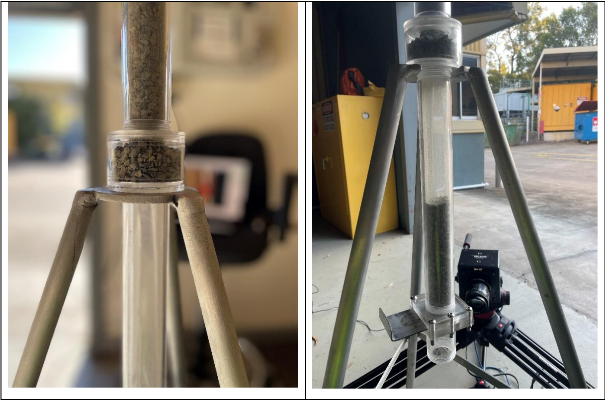
Figure 2: View of the apparatus built at CSIRO to investigate the flowability of rock-like fragments in pipes
