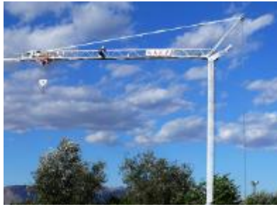
Figura 19: Grúa torre SELF-ERECTING Hidráulica H 25
