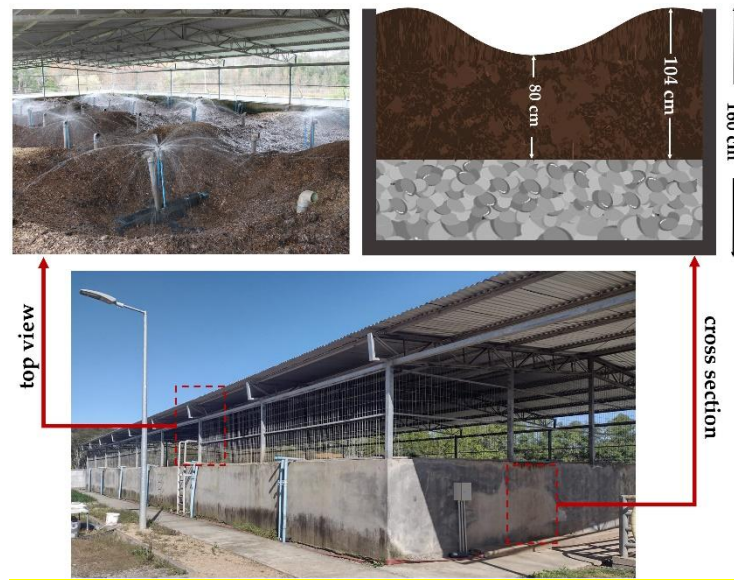
Figure 4.1. Schematic representation of the active layer.
