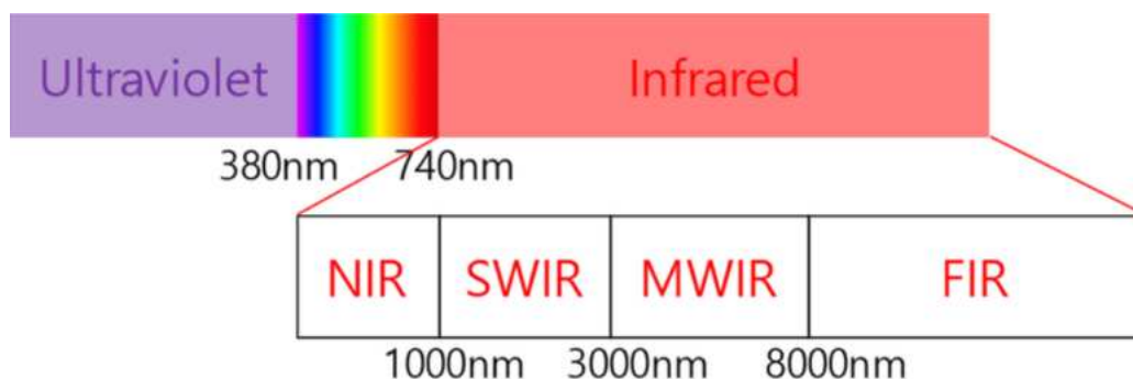
Figura 3.1: Desglose del espectro IR, las secciones corresponden a NIR( Near Infrared ), SWIR( Short Wave Infrared ), MWIR( Mid Wave Infrared ) y LWIR( Long Wave Infrared ) [1].
