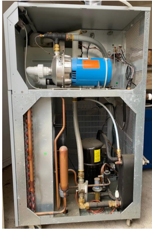
Figura 3.17: Componentes del Chiller ThermoFlex10000.
