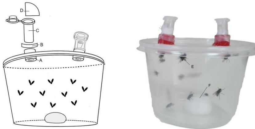
Figure 1. Outline the components of the fumigant test device, showing the sample test tube lid (A), the tulle mesh (B), the Eppendorf tube (C), and the filter paper (D).
