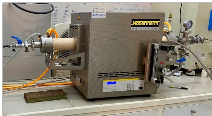
Figura 4.9 Horno 3: Mufia tubular Nabertherm.
