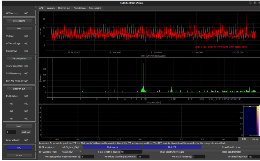
Figure 4.5.2: Display of the counts and frequencies detected by the APD seen on the CODE control program, with a resolution of 0.1 Hz.
