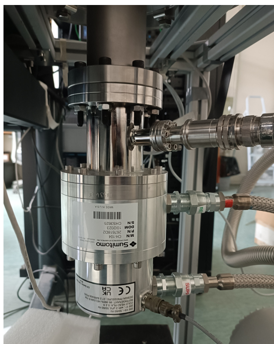
Figure 4.7.1: Cold head connected at the bottom of the vacuum chamber.
