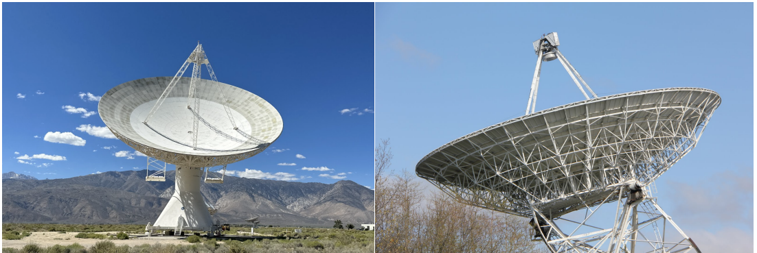
Figure 3.1: Radio telescopes providing the long-term monitoring used in this thesis. Left: the OVRO 40-m telescope (15 GHz) located in Owens Valley, California (USA). Right: the UMRAO 26-m telescope (14.5 GHz) located in Dexter, Michigan (USA).
