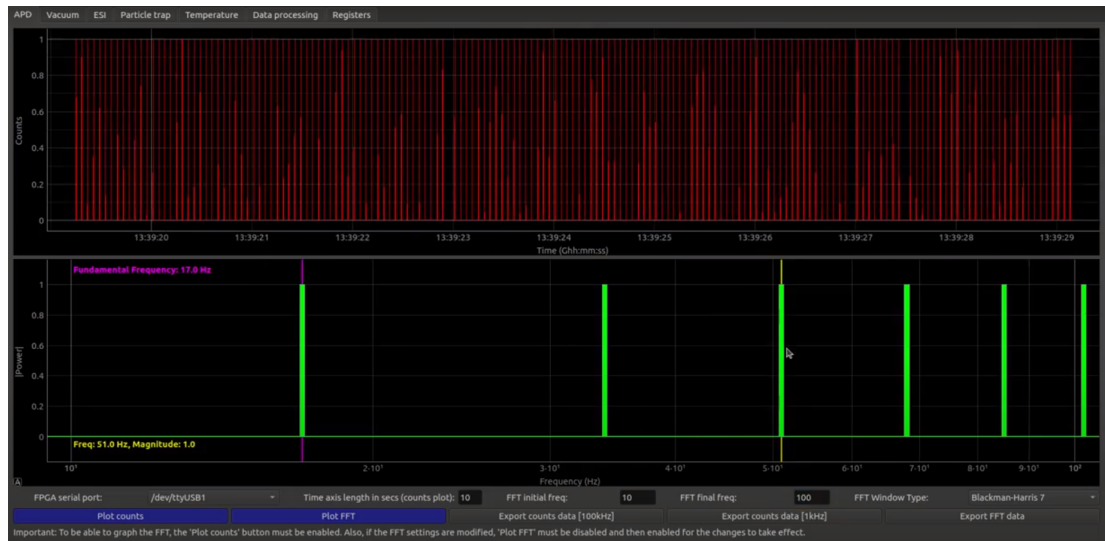
Figure 3.3.6: CODEs control software. The red graph shows the counts sent by the APD with a 500 Hz sample rate. The green graph shows an FFT of the APD counts with a 0.1 Hz resolution and a maximum frequency of 50 kHz.
