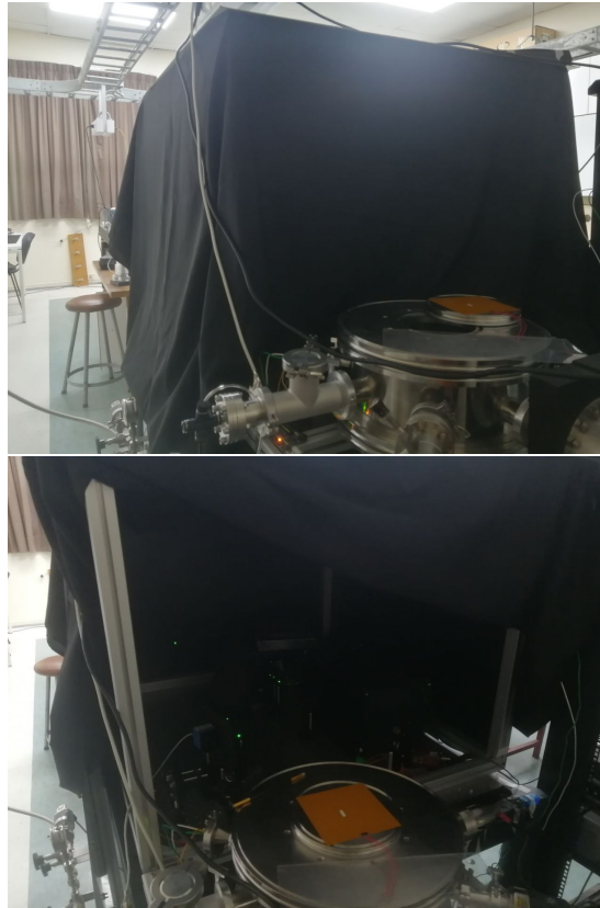
Figure 3.1.7: The code experiment as seen with its enclosure, since the chamber itself is closed, only the viewports are covered with the enclosure to ensure only the light from the optical system reaches the APD/camera system.
