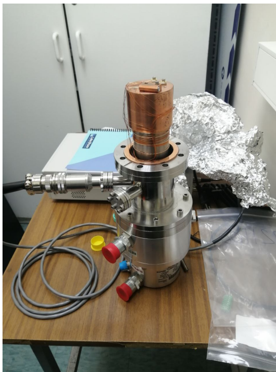
Figure 6.2.1: The CODE experiments cold head, it is attached from the top with a custom-made adapter that allows for the connection of the trapping system inside.
