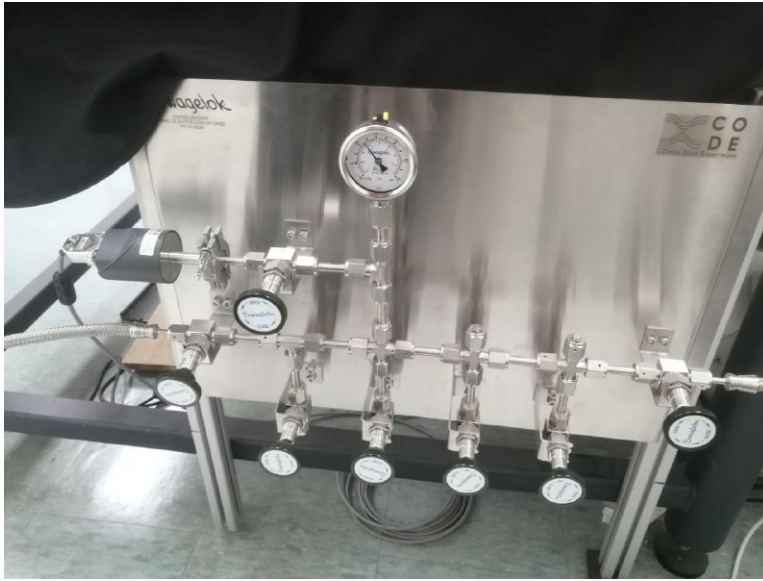
Figure 3.1.8: The CODE gas line system, we can see 4 gas lines for additional connections in the bottom and to the left is the argon line, the connection on the right goes to the vacuum chamber.
