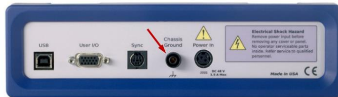
Figura 34 Chassis Ground del potencióstato Gamry [29]
