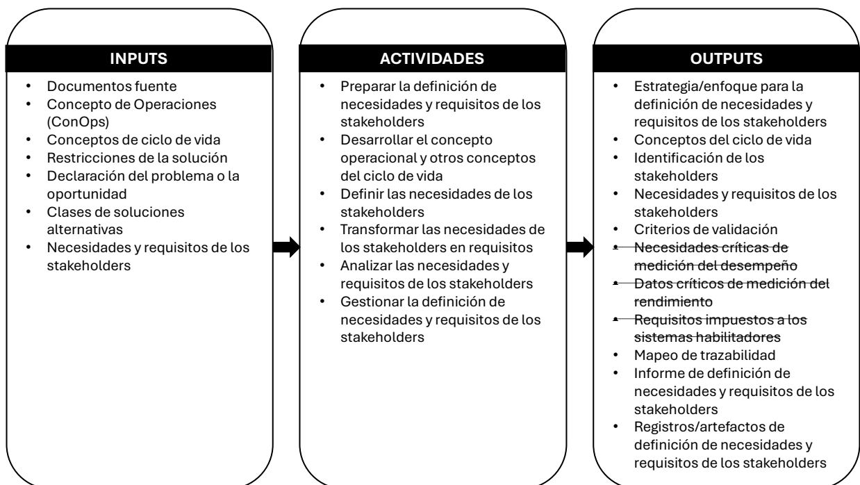
Figura 4: Diagrama IPO de Stakeholders Needs and Requirements Definition Process. Adaptado de Systems Engineering Handbook (INCOSE, 2023, p. 108)
