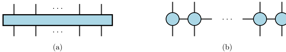
Figure 4.20: (a) Tensor O_{\alpha_1 \dots \alpha_n \beta_1 \dots \beta_n} at the LHS of Equation (4.15) and (b) its MPO factorization at the RHS.
