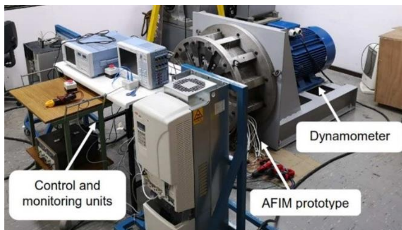
Fig. 3.11 Test bench and equipment used to operate the AF-MRIM prototype.
