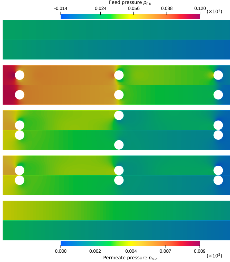
Figure 2.9: Pressure drop in the region [3, 12] \text{ mm} \times [0, 1.48] \text{ mm} . From top to bottom: cases (C.1), (C.2), (C.3), (C.4) and (C.5). Simulation conditions: u_{\text{in},f} = 0.1 \text{ m/s} , u_{\text{in},p} = 0.01 \text{ m/s} , \Delta P = \Delta P_2 .
